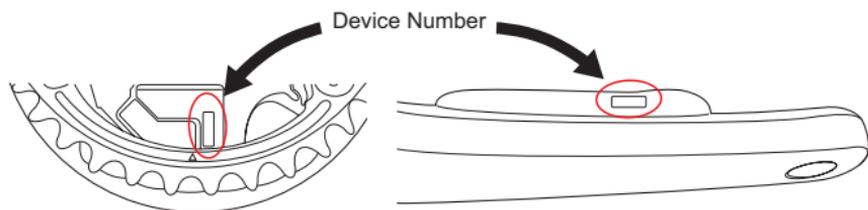
Check that the device numbers are those of the pedaling monitor sensors being used.
