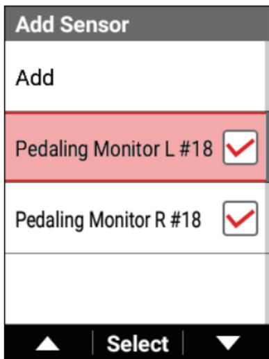
The sensors with check boxes selected are added to the sensor list. Clear the check mark for any sensor that does not need to be added to the sensor list in advance.
