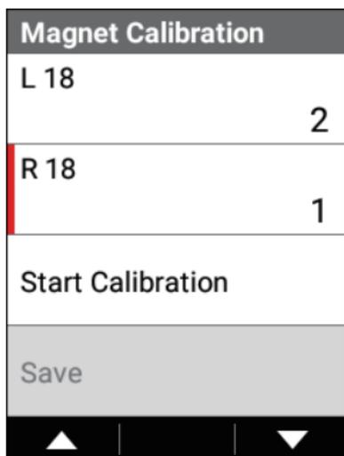
If the counter is not incremented, readjust the magnet position.
