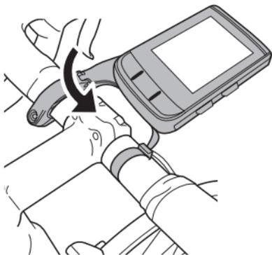
Turn the device all the way until it is as shown in the figure below and then lift it up slowly.
