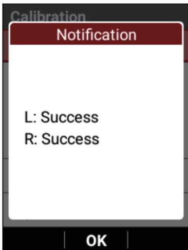
If "Failure" is displayed, calibration may have been performed when the crank is in an unstable state such as when it was moving. Perform zero point calibration again when the crank is still.
