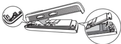
When disconnecting the lithium-ion battery cable, please hold and pull the connector without pulling the cable part.
