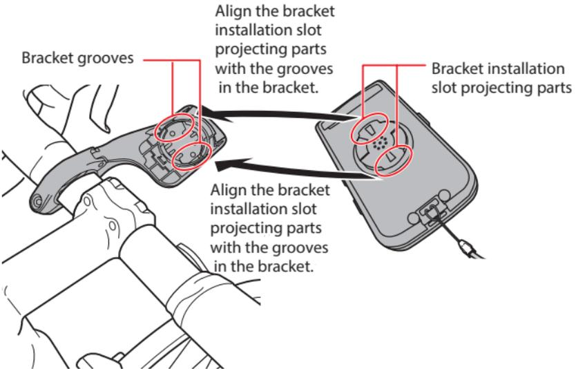
When the projecting parts are aligned with the grooves, the device will be at the angle shown in the figure below. Securely fit the two protruding parts into the grooves.
