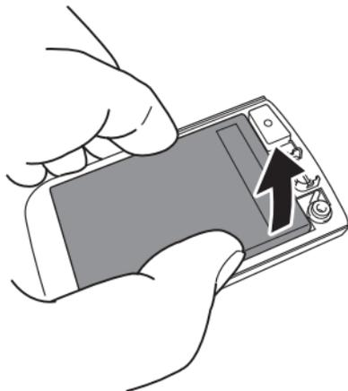
**4 Remove the lithium-ion battery from the back cover.**
