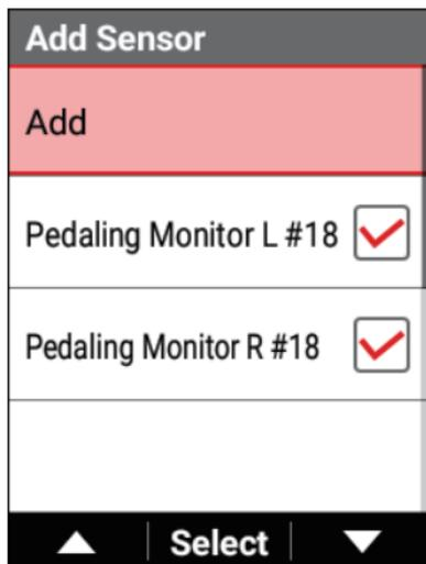
The left pedaling monitor and right pedaling monitor for which you selected the check boxes are added to the sensor list.
