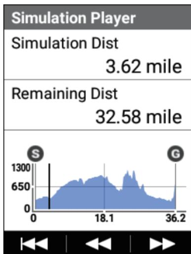
Each press of the [→] button moves forward by a distance of 10%, and each press of the [Confirm] button moves back by a distance of 5%.
