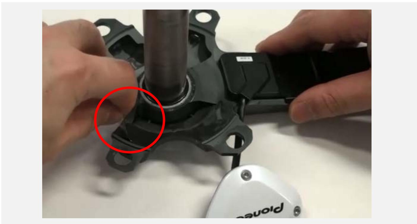
Do not allow the sensor cable (circled in yellow) to lie on the outer, lower area of the spider arm.
