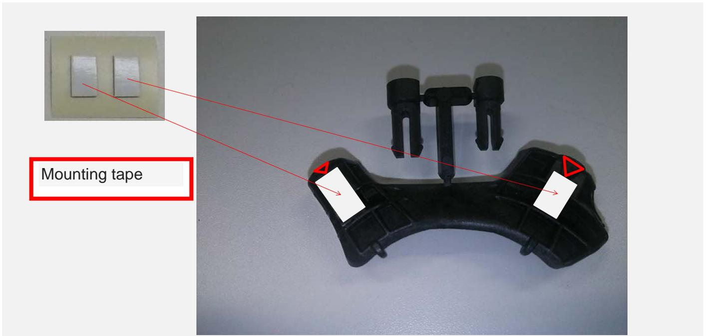
Disconnection of the adapter base body and the fixing pin
