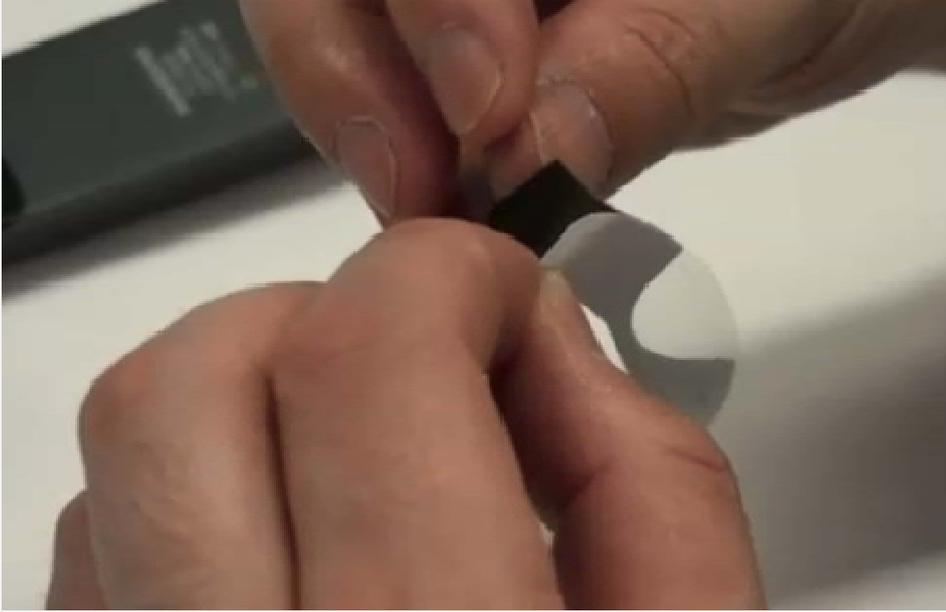
Holding the double sided tape by the transparent in the center, attach it to the spider arm.
