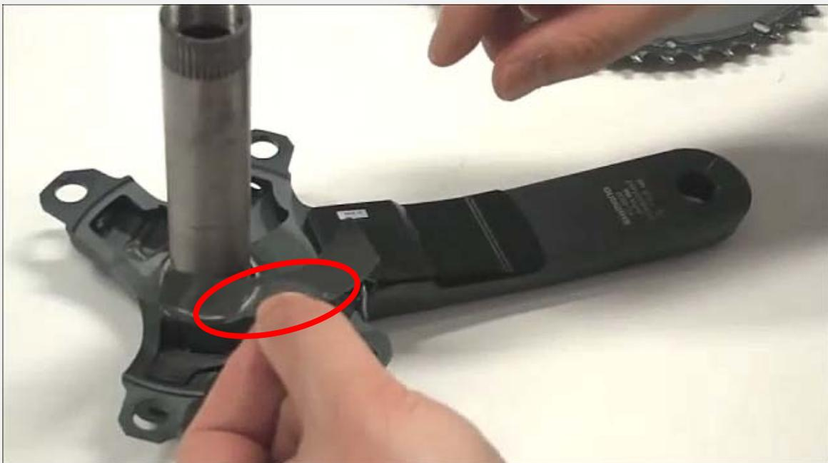
Adjust the position of the curved portion of the adhesive tape to fit the position of the blue line (below)
