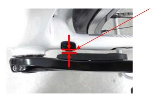
For the left and right sides, try to affix the magnet so that it is within 1.5mm and 10.7mm of the sensor. If this is not possible on the Chainstay, try the Seat Tube (right photo) or the Down Tube.
