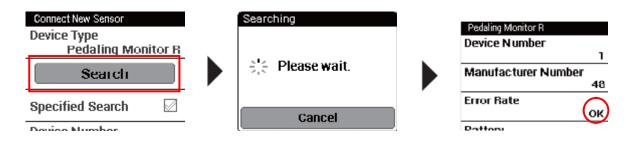
Pairing of the right transmitter is completed. Pair the left transmitter in the same way.
