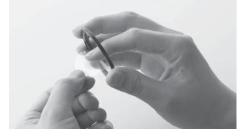
2 Adjust the orientation of the magnet rings so the opposite side of the "L" and "R" marks (diagram below) cover the screw part on the attachment.
