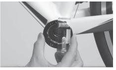
• Attach the magnet rings so the screw part on the attachment points downward.
