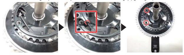
4 Put grease on the chainring bolts and insert them into the bolt holes and temporarily install the chainring adapter on the chainring.
