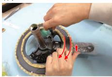
· Refer to the instruction manual for the crank set you are using for the torque at which to tighten the chainring bolts.
