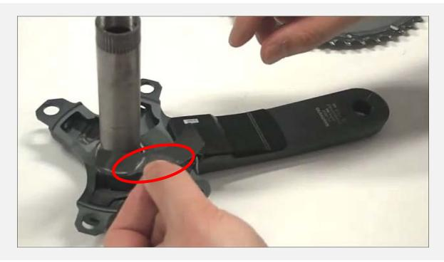
Adjust the position of the curved portion of the adhesive tape to fit the position of the blue line (below) Be careful not to cover the portions marked with Red lines.(below)
