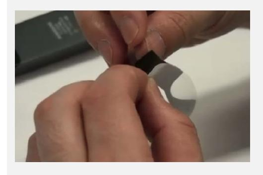
Holding the double sided tape by the transparent in the center, attach it to the spider arm.
