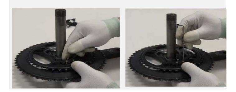
Use a tool to measure the torque when you tighten the screws.
