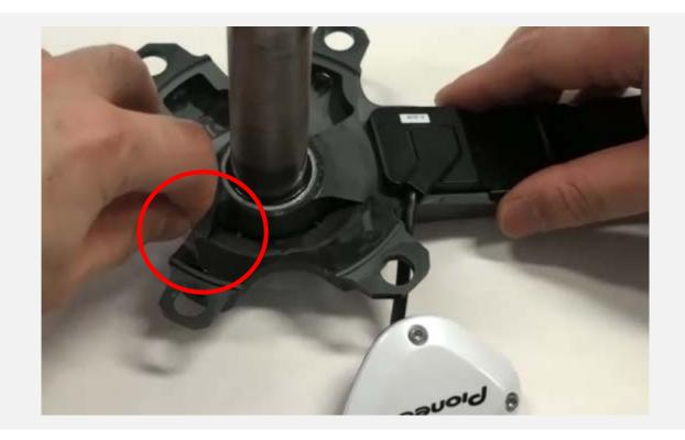
Do not allow the sensor cable (circled in yellow) to lie on the outer, lower area of the spider arm.
