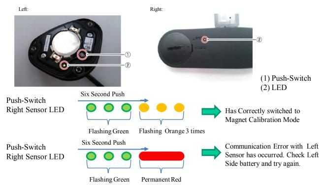
Rotate the cranks slowly and evenly at around 30rpm. Check that both LEDs flash GREEN once per revolution. If either LED shows RED, the rotation is too fast. Rotate slowly at 30rpm (2 seconds per revolution). If the LED does not light at all, it is not detecting the Magnets. (Too far away or not passing the Magnet.) Return to Step 1 and reattach the Magnets
