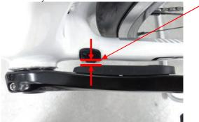
The Magnet Sensors on each side should be between 1.5 and 10.7mm from the Magnets.
