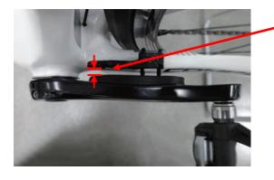
Ensure that the Magnets are between 1.5mm and 9.6mm from the sensors.
