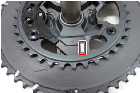
Right side: Junction box
