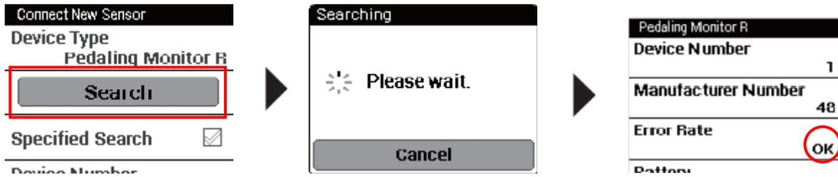
Pairing of the right transmitter is completed. Pair the left transmitter in the same way.
